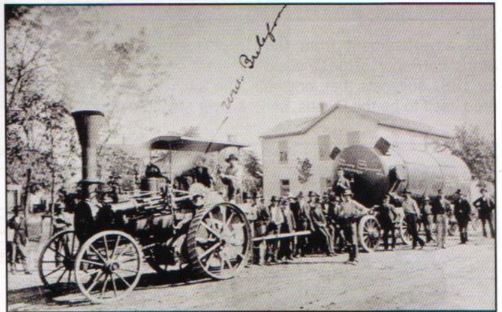
This Ritchie & Dyer engine was photographed on Broad Street in Middletown around 1890. Characteristic of the early Ritchie & Dyer engines, it is virtually an Owens, Lane & Dyer. Courtesy Middletown (Ohio) Historical Society
