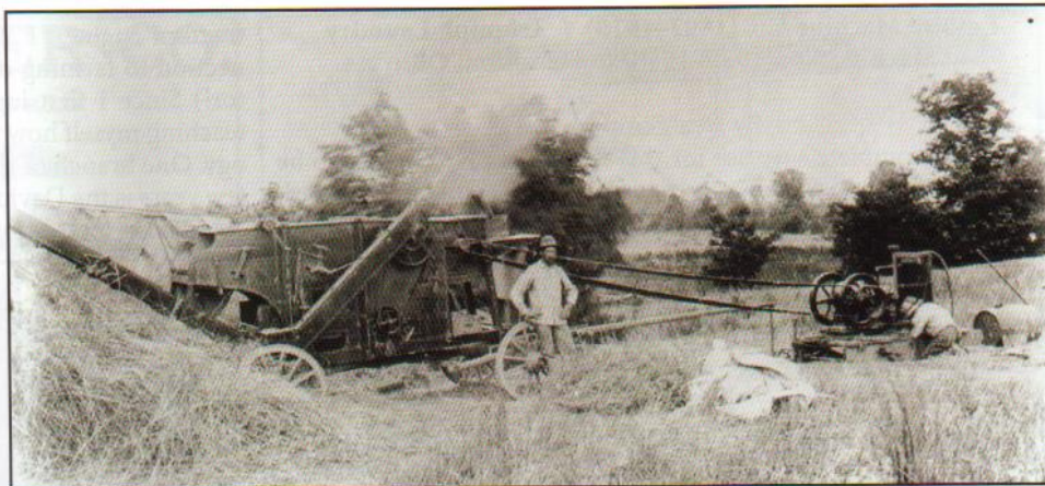
A Hamilton gasoline engine, built by the Advance Manufacturing Co., has enough power to run this threshing machine. Courtesy George C. Cummins Collection of the Lane Public Library of Hamilton, Ohio
