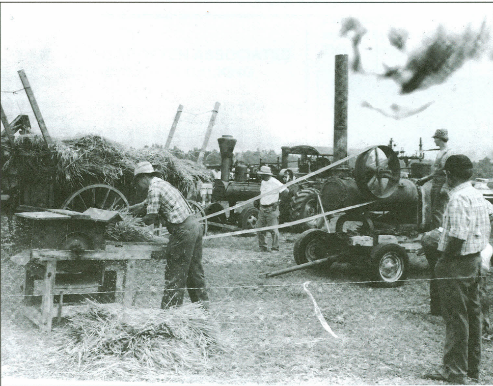
Besides steamrollers, the Harrisburg Car Mfg. Co. also built skid, portable and traction engines. This 5x8 skid engine, mounted on a wagon running gear, was built in Harrisburg, PA and spent its working life powering a basket factory in Delaware. It is shown powering a groundhog thresher at the Eastern Shore Threshermen show near Federalsburg, MD. Photo by Brenda Stant.
