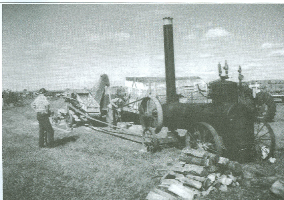
Woodgum 6 HP portable shown with all wood Adams corn sheller, patented November 1904. Under power at the 1992 Antique Engine & Tractor Association Inc. Show in Atkinson, Illinois.
